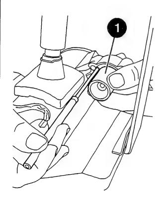
Disassembling bearing-end plate
